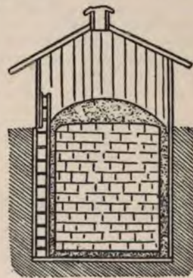
Fig. 253. Ice-house built below surface of ground.
